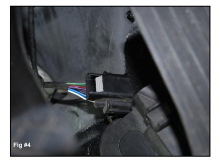
Step 5- Slide the Sprint Booster into the OEM harness plug first, be sure to take care doing this as you don't want to harm the pins in the connector. Once firmly connected, the factory harness slider mentioned earlier will pop back out. On a car with some spirited miles the slider may need some cleaning to free its movement.
