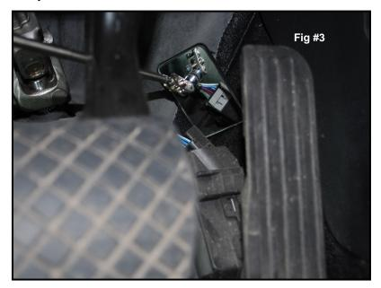
Step 4- Once the slider is fully in place, pushed into the connection, give the connection a good pull to separate the connector from the pedal. The slider will remain in the downward position until reconnected to the Sprint Booster. See Fig #4 to show how the slider will look while disconnected.
